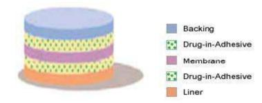
The Multi-layer Drug-in-Adhesive is similar to the Single layer Drug-in-Adhesive in that the drug is incorporated directly into the adhesive. However, the multi-layer encompasses either the addition of a membrane between two distinct drugin-adhesive layers or the addition of multiple drugin-adhesive layers under a single backing film.
